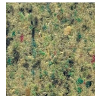
2,5 mm linoleum + 1,5 mm recycled foam
